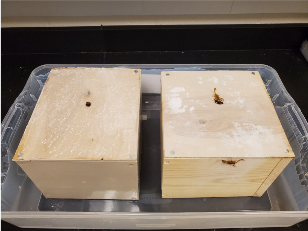
Figure 1. The testing arena and wooden structures used in this tests; the structure coated in Averzion on the left and the untreated control on the right. Pictured is a dead cockroach placed on each as a food item for the scorpions.
